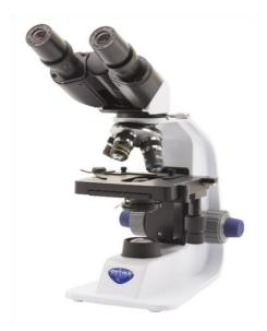
Binocular microscope, 400x, rechargeable, N-PLAN objectives
