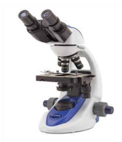
Binocular brightfield microscope, 600x, PLAN, multi-plug
