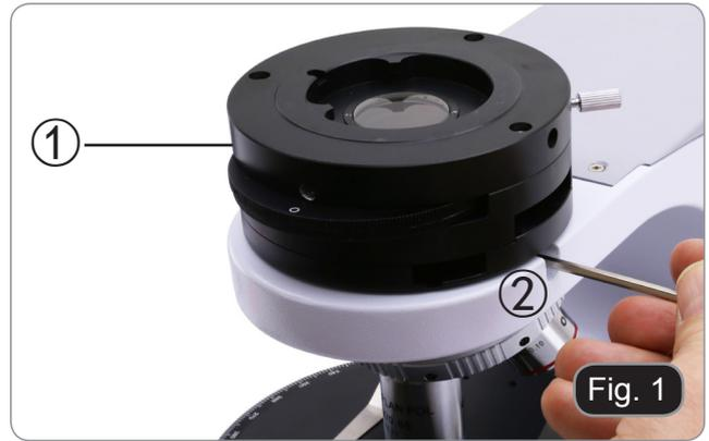
2. Insert the optical head on the Bertrand lens and lock the locking screw with the provided Allen wrench. (Fig. 2)
