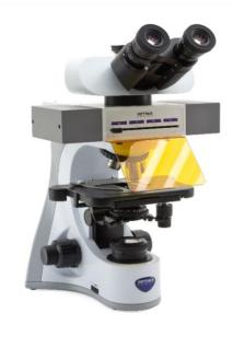
Trinocular LED fluorescence microscope, 1000x, IOS W-PLAN objectives
