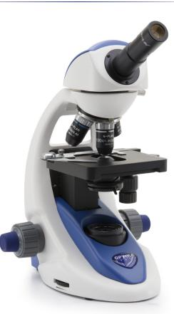
Monocular microscope ideal for teachers and secondary schools, with four N-PLAN objectives (1000x), FN 18 high eyepoint, finite optical system, coaxial focusing, mechanical stage, Abbe condenser and powerful, uniform, white color temperature 3 W **X-LED**<sup>2</sup> illumination. Slim and easy to carry, yet sturdy and resistant, it is equipped with all the main controls to start learning how to use an advanced microscope and with long lasting LED illumination to provide over 20 years of use
