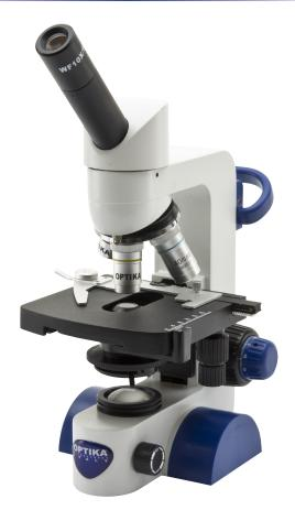
Cordless, modern monocular microscope ideal for students and mainly primary schools with achromatic lenses (400x), FN 18 eyepiece, finite optical system, coaxial focusing, StagErase™ mechanical stage, Abbe condenser and 1 W LED illumination with rechargeable batteries (not supplied). Slim and easy to carry, it is equipped with arm/wrist rest support to reduce the fatigue during use and long lasting LED illumination to provide over 20
