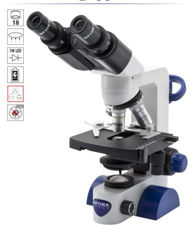
Cordless, modern binocular microscope ideal for students and mainly primary schools with achromatic lenses (400x), FN 18 eyepieces, finite optical system, coaxial focusing, StagErase™ mechanical stage, Abbe condenser and 1 W LED illumination with rechargeable batteries (not supplied). Slim and easy to carry, it is equipped with arm/wrist rest support to reduce the fatigue during use and long lasting LED illumination to provide over 20 years of use.
