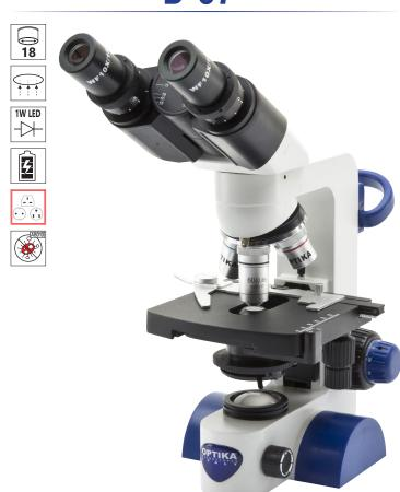
Cordless, modern binocular microscope ideal for students and mainly primary schools with achromatic lenses (600x), FN 18 eyepieces, finite optical system, coaxial focusing, StagErase™ mechanical stage, Abbe condenser and 1 W LED illumination with rechargeable batteries (not supplied). Slim and easy to carry, it is equipped with arm/wrist rest support to reduce the fatigue during use and long lasting LED illumination to provide over 20 years of use.
