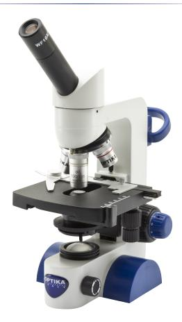
Cordless, modern monocular microscope ideal for students and mainly primary schools with achromatic lenses (600x), FN 18 eyepiece, finite optical system, coaxial focusing, StagErase™ mechanical stage, Abbe condenser and 1 W LED illumination with rechargeable batteries (not supplied). Slim and easy to carry, it is equipped with arm/wrist rest support to reduce the fatigue during use and long lasting LED illumination to provide over 20 years of use.
