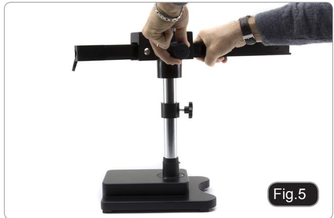
5. Install the head holder. Head holder can be installed in several ways according to specific need of the user.
