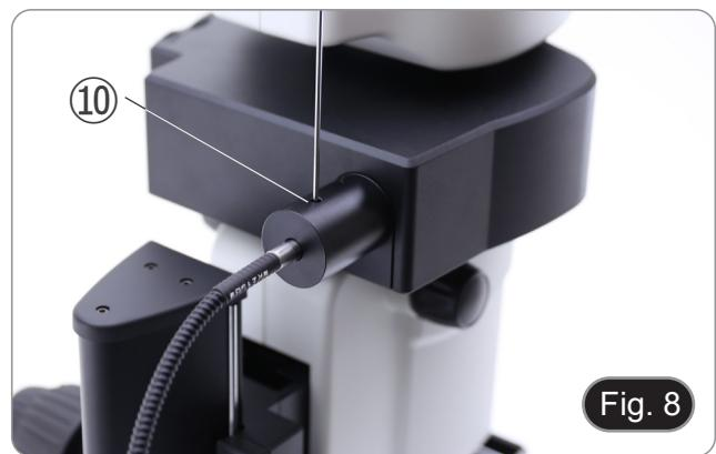
16. Insert the other one end of the light guide into the light source.
